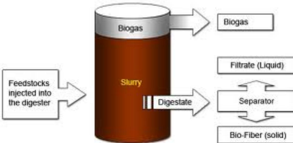
Basic Anaerobic Digestion Process
