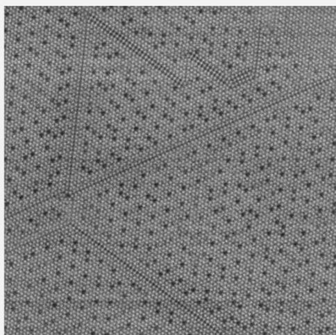
The *ab* planes of M2 shows some very unusual structural features of a defective M2 phase: point defects corresponding to missing Te sites which are visible as dark spots, and two-dimensional (planar) defects visible as series of intersecting “zippers”.
