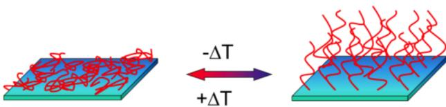
The thermal response of PNIPAm is used for membrane de-fouling and tissue engineering.
