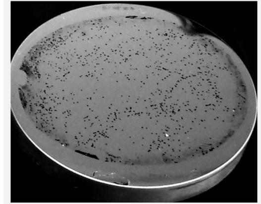
Electrochemically-induced pitting of aluminum deposited on a silicon wafer
