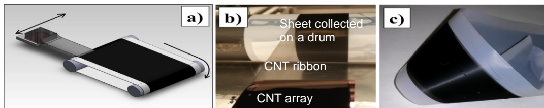
Fig. 2. CNT sheet assembly process: a) schematic representation; b) picture of CNT sheet fabricating process; c) picture of CNT sheet (100 layers) supported by a Teflon film.
