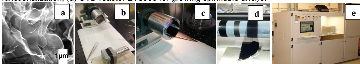
Fig. 5. Nanotube thread and sheet spinning and drawing at UC: (a) pristine 3D graphene; (b) ring spinning machine; (c) close-up of ring head invention at UC with four substrates spinning at once; (d) drawing ribbon for functionalization; (d) CVD reactor ET 3000 for growing spinnable arrays.
