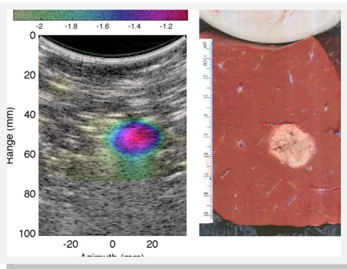
Echo decorrelation imaging from a 4 MHz, 128-element curved linear array with corresponding section of RFA-ablated *ex vivo* liver.
